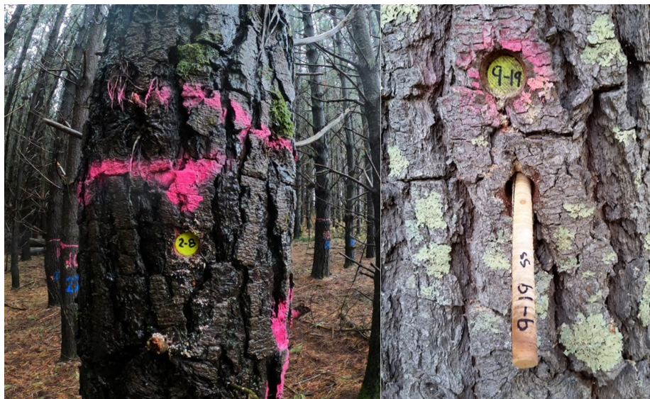
Figure 2: Twenty trees were selected as sawlogs. Plugs were inserted in the outerwood core sampling hole to assist in identifying individual butt logs in the log yard, and on three trees per site full radius cores were taken for SilviScan analyses.
